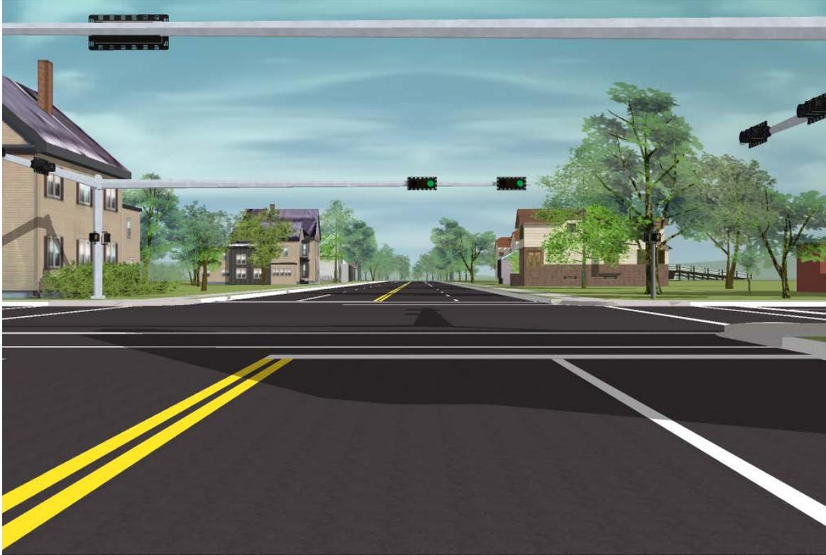
Figure 2. Example of a standard marked crosswalk at 50 ft.
